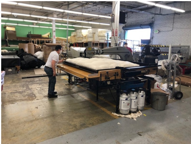
A worker uses a special machine to insert buttons in a futon.
