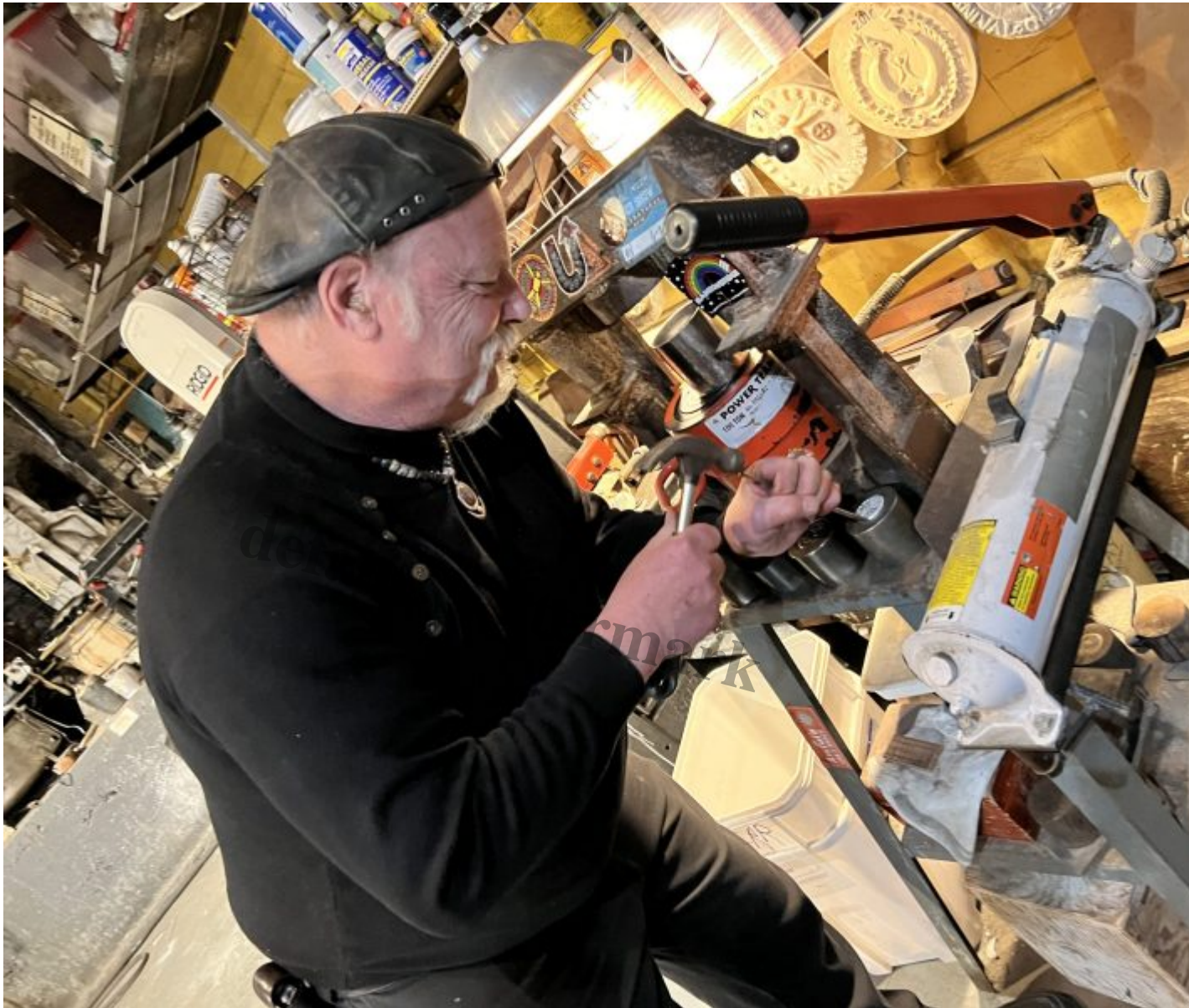
Macchiarini demonstrates the 100-ton press that was used at Burning Man to recycle aluminum cans into coins representing the festival's theme.
